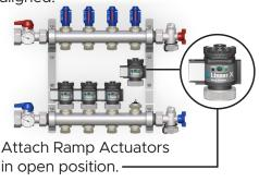
2. Attach Linear-X into the Ramp Actuators front lower groove.
